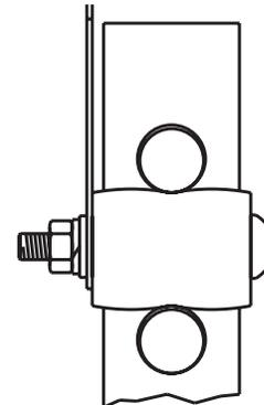
**CAUTION** If pipe sealant is used on threads, the degree of resistance between mating parts is less, and there is an increased chance for cracking the heat exchanger fittings. Do not overtighten.
